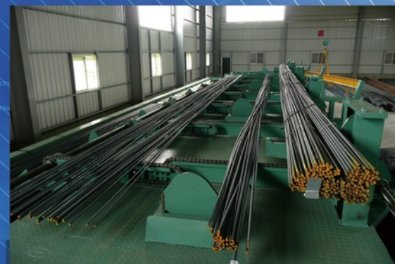
● 鋼筋舉昇機構 Steel Bar Lifting Machine
